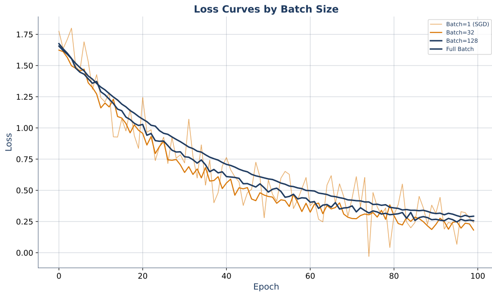
Figure 49: Loss curves for different batch sizes. Smaller batches show more noise per step but often generalize better; larger batches are smoother but can get stuck in sharp minima.
