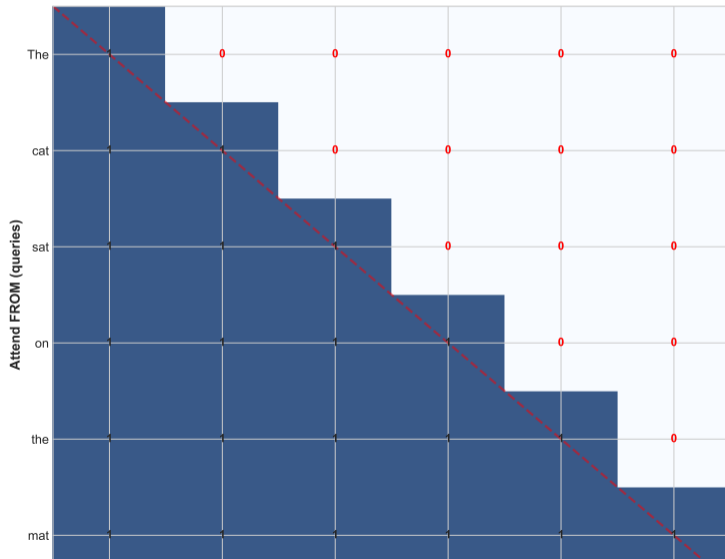
GPT Causal Mask: Lower Triangular (No Future Peeking)
